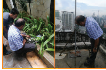
To conduct electrical safety earth resistance test at a condominium - 639 Residence, Jalan Scotts -
